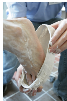
Casts were used to create a series of one off prototype insoles for testing. Below, prototype insole in red
